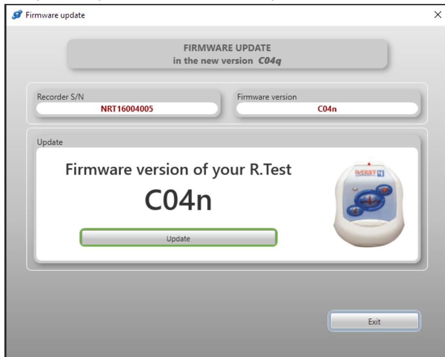
After viewing the window, the user is prompted to click the 'Update' button. You must not disconnect the recorder from the PC during the update as it will be damaged.
